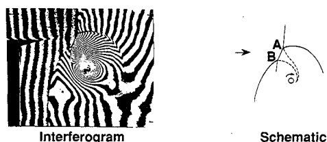
Fig. 10 Experimental study of strong shock-vortex interaction (from Ref. 11).
